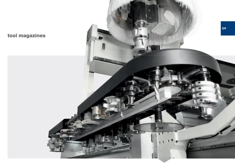
The machine is always equipped for any machining using the TRC chain magazine with 48 locations available for large and double-profile tools.
