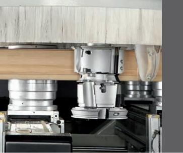
Prisma allows machining up to 10 degrees below the horizontal axis.
