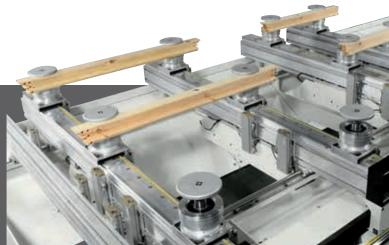
Workpiece loading and unloading is easy and ergonomic. They are automatically carried to the machining zone to prevent any kind of collision thanks to total worktable management.
