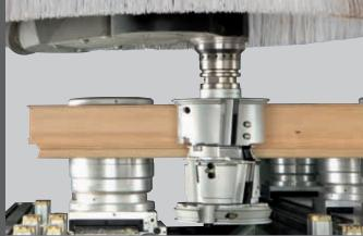
All versions of SCM worktables use common accessories The H110 worktable allows maximum freedom of movement and always offer ideal hold-down to provide top quality with tools and even use of "double-profile" tools. finishing even with heavy duty stock removal.
