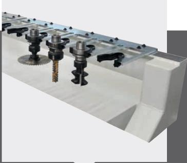
To have the most tools available, the rack magazine may have up to 12 locations, using the items present on the machining head.
