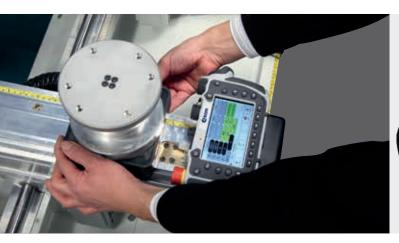
In the "Pilot" version positioning is guided and controlled by the workpiece program. Magnetic sensors detect the correct position of all components, eliminating the risk of collision.
