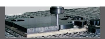
The directly machined worktable guarantees lasting absolute precision and perfect flatness thanks to its high level of rigidity. Also ideal for machining plastics, resins and light alloys.
