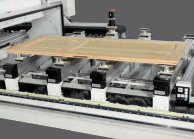
Matic is the fully automatic worktable ideal for machining solid wood. Complete set-up in seconds, all bars and supports moving simultaneously, each driven by an independent motor. The many technical devices give this table lasting safety and reliability.
