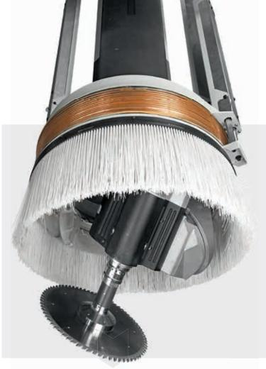
Compact and powerful, the Prisma head can use any type of tools, even large tools for intensive machining operations typical for door and window frames.
