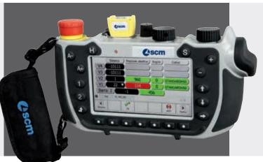
Fast operations that do not require any further checks; the display on the mobile console shows the position for each element and provides a real-time view of all movements until the correct position is reached.
