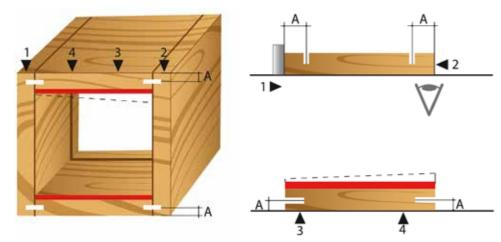
**Perfect finish,** drilling on the top side allows external part of the panel to be referenced, hiding any squaring defects of the piece.
