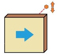
No panel loading errors with the Y congruence sensor that checks that the size of the panel inserted matches the size programmed.
