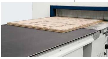
High productivity: the pusher moves the processed work pieces on the unloading belt and simultaneously cleans the work table while the new panel to be machined is loaded.
