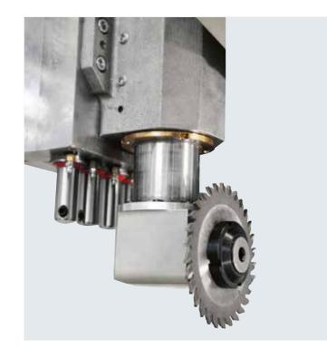
Easy cutting and grooving operations along X and Y direction thanks to the 0°-90° blade unit.
