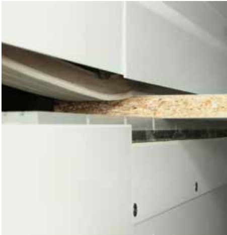
Smooth and precise panel movement thanks to the pressure belt.
