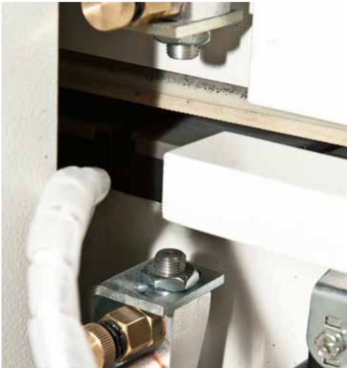
ANTI-ADHESIVE UNIT FOR FREE SPACE 1-AA Free space for anti-adhesive unit. To avoid glue deposits on the top and bottom surfaces of the panel.
