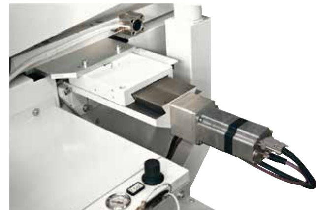
Entry guide, manual (std), pneumatic or NC versions (opt)
