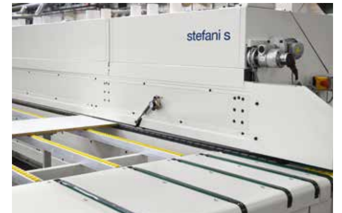
Automatic infeed system and single-belt/multi-belts transfer for the machine integration with upstream and downstream handling equipment (opt)
