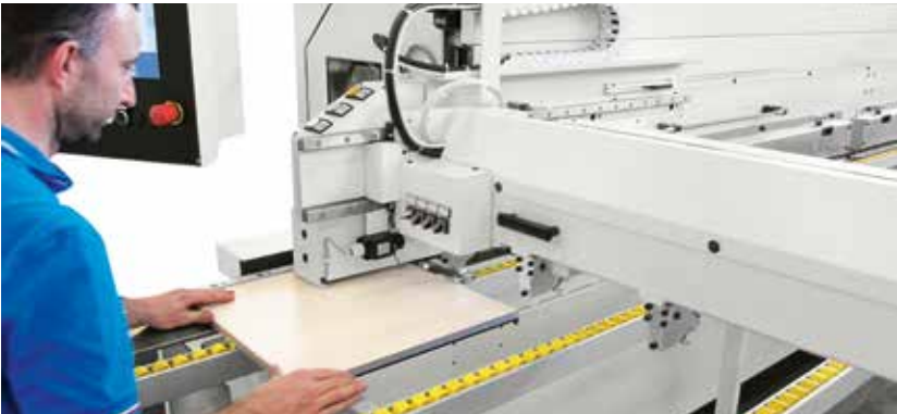
Manual infeed device It makes easier the introduction of panels already squared
