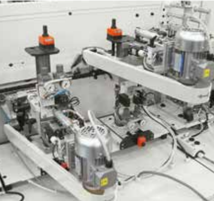
Sanding unit for chamfers/radii.
