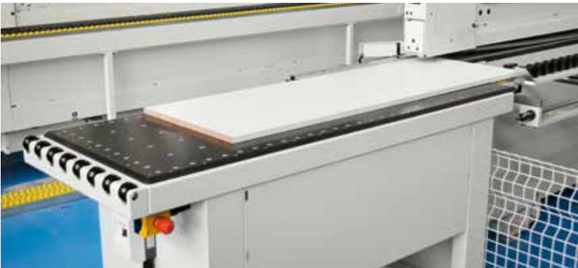
Air cushion table Easy and fast movement of panels in the loading area with the air cushion table.
