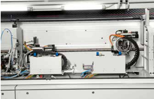
CORNER ROUNDING UNIT WITH 2 POWER ASSISTED MOTORS
