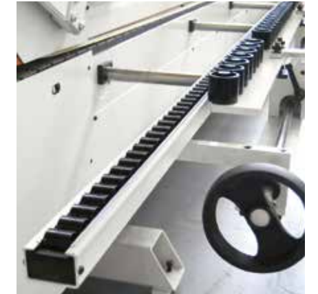
Counter shoulder for narrow panels, solid wood or softforming (opt)
