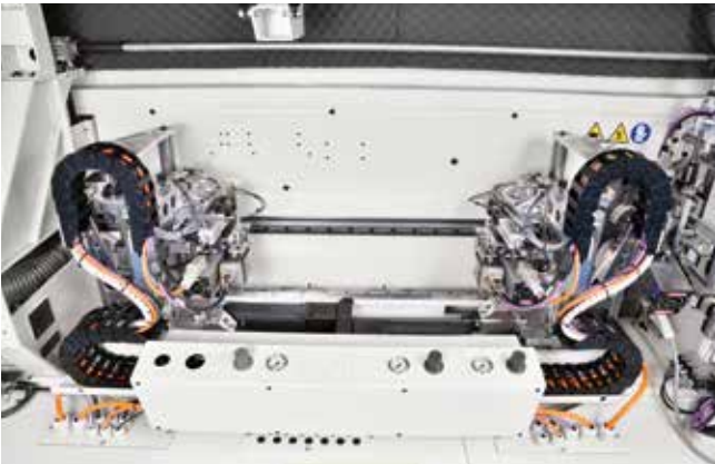
CORNER ROUNDING UNIT WITH 2 MOTORS
