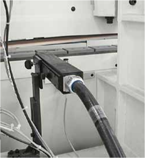
Inkjet printer for the marking of the panel in the upper or lateral surface.
