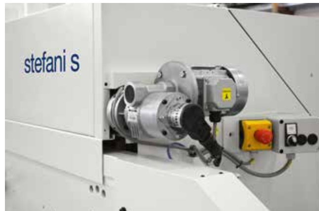
Top pressure device with NC movement (std)
