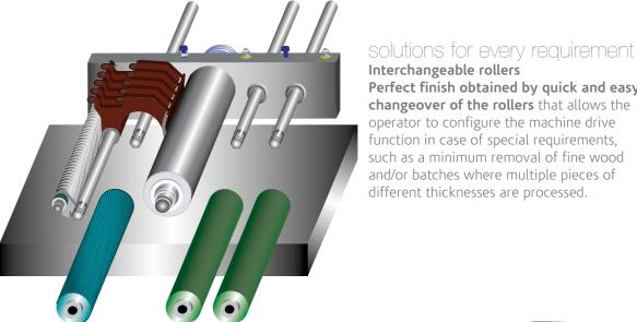
Perfect finish obtained by quick and easy changeover of the rollers that allows the operator to configure the machine drive function in case of special requirements,
