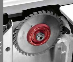
Blade diameter: 120 mm (160 mm for class si x)
