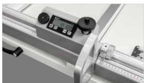
Electronic readouts on the squaring stops The stops can be easily read
