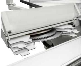
Blades-holder drawer integrated in the machine's frame
