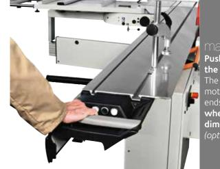
Pushbuttons integrated in the sliding carriage
