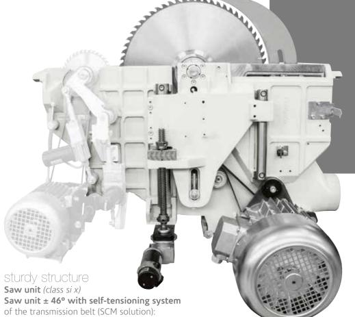
The saw blade lifting is carried out sectors in a crescent shape to ensure reliability over time
