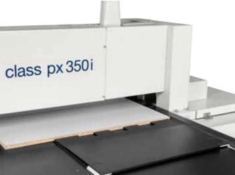
Immediate and precise positioning thanks to the powered and programmed rear stop.
