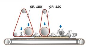
After planing, the surface of the panel needs only a slight degree of finishing. This can be done with a 150 grit sanding belt using a single operating unit or a 180 grit sanding belt using two operating units.
