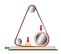
Calibrating / sanding with roller and sanding with pad
