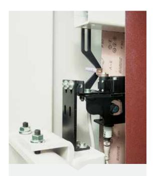
Belt oscillation controlled by an electronic photocell
