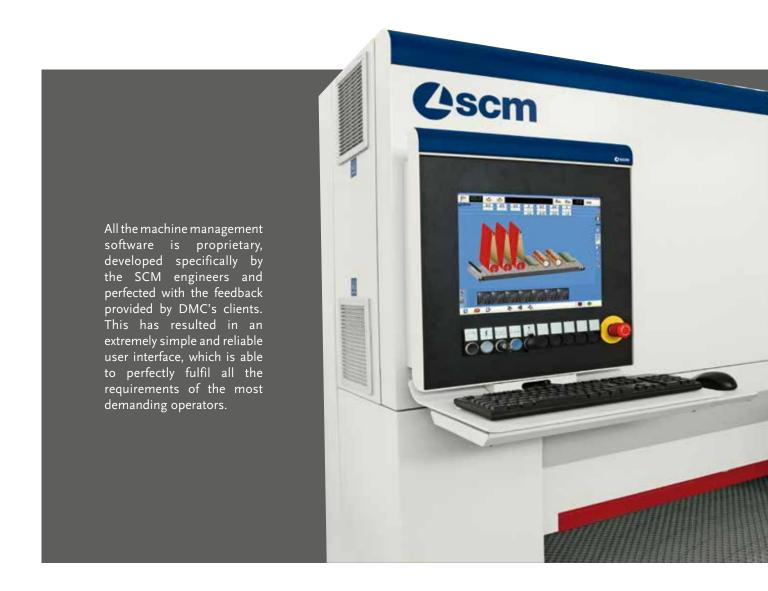
The "Pro-Sand" control, fitted as standard on all the DMC System sanders, is used to set all the operating parameters on the touch screen, and to check in real time the correct operation of the machine.
