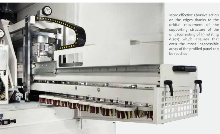
The rugged brushes ensure that the sanding operation will result in the creation of surfaces of the highest quality. This is facilitated by devices which control the oscillation of the roller and regulate the inclination of the strips, allowing the abrasive action to be standardised.
