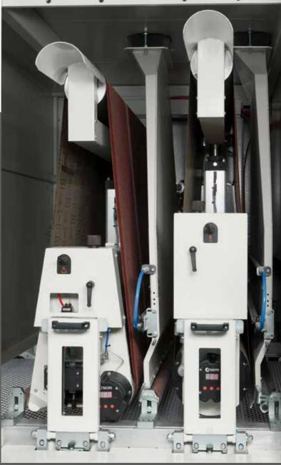
The new fast locking system used to fasten the units to the base and the digital display of the operating quota render machine settings extremely fast and precise.
