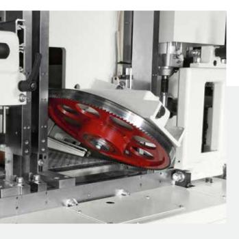
The innovative "saw blade" unit allows users to recreate the irregular surface effect produced by using a bandsaw. The ability to regulate the depth of the blade cut, and the rotation speed of the blade, enables the user to control the depth and distribution of the cuts, making it possible to choose the kind of finish users wish to create every single time.
