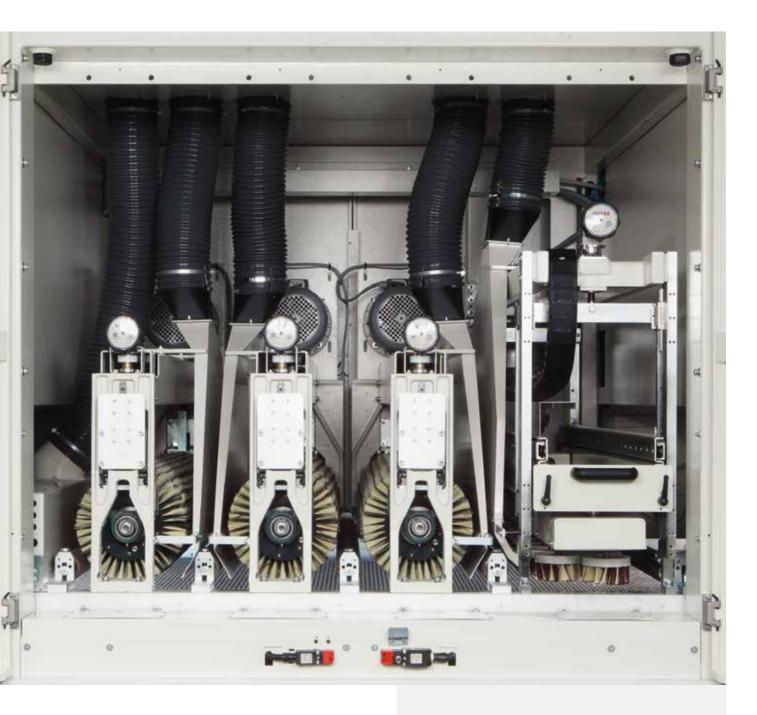
The ideal configuration for creating finishes for assembled doors, window frames and profiled elements in general (strips for frames, door and window frames, trims, matchboards, skirting boards, etc.), regardless of whether they are rough or painted.
