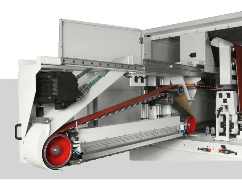
The compact internal crossbelt unit can be placed in any position inside the machine, according to the specific machining requirements of the client. The innovative unit side extraction system on telescopic guides allows a single operator to replace the sanding belt very easily, and it facilitates the regular cleaning and inspection activities. The unit is fitted with the "EPICS" electronic sectional pad, power driven rotating blowers to clean the sanding belt and motor driven by inverter.
