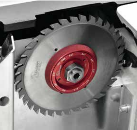
expandable scoring blade Manually expandable with variable thickness from 3,5 to 4,5 mm (blade diameter: 160 mm).
