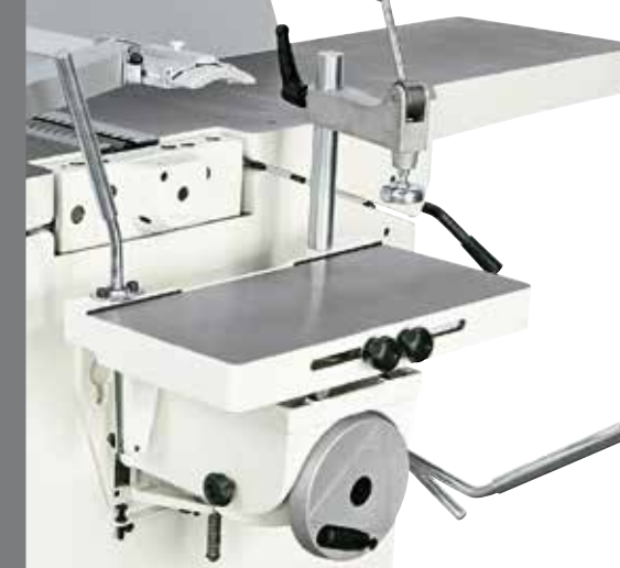
cast iron mortiser Drilling holes and mortises are easily carried out. Complete with exhaust hood, 120 mm diameter and 16 mm chuck.
