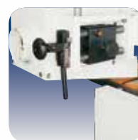
Belt Tensioning Device practical to use
