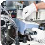
Interchangeable Glue Pot also for PU gluing
