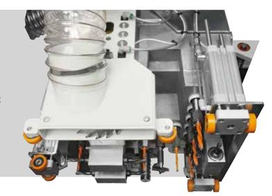
**Very short machining cycles** and **zero dead times** for set-up operations; the drilling head with 18 independent spindles (12 vertical, 4 horizontal along X axis, 2 horizontal along Y axis) and blade along X axis cover the whole surface of the panel to be machined:
