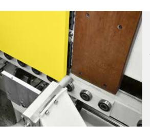
Highly versatile, the programmable side reference stop lets you machine pieces with dowels already inserted or with routing already carried out.
