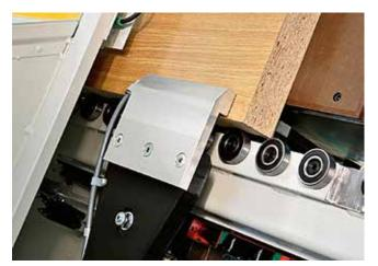
Maximum piece stability and high machining quality, with the mobile clamp with floating opening that does not require any adjustment and the Bakelite non-scratch table that guarantees high machining quality also for panels with delicate surfaces.
