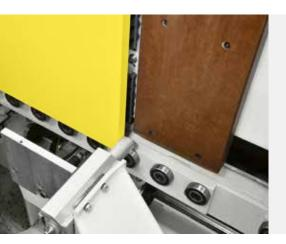
**Highly versatile:** the programmable reference stop allows the machining of pieces with dowels already inserted or with routing already executed.
