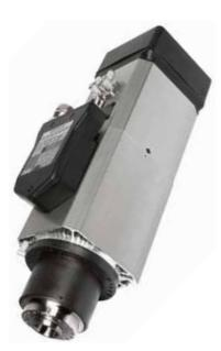
**Highly functional and reliable:** the 6.6 kW electrospindle with HSK63-F taper and rotation speed up to 24,000 RPM, is the ideal solution for local routing operations on various types of panels. Positioned on the upper head it can be used for blind and through routing.
