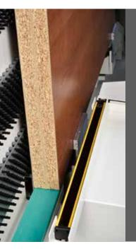
**Maximum** productivity: the transport system with 2 independent clamps can handle panels up to 95 mm thick and 1300 mm heigh, at a speed of 70 m/min.
