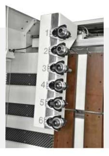
**Flexible:** the 6-position tool changer ensures that all the tools necessary to complete all the machining operations of the piece of furniture are available.
