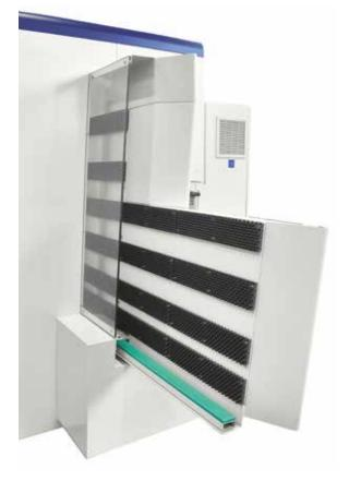
**Ergonomic:** the lateral supports allow operators to comfortably load and unload panels up to 3050 mm.
