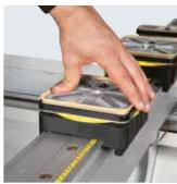
It is possible to add or remove vacuum pods or clamps with a simple movement of the hand; the number and the position are automatically detected.
