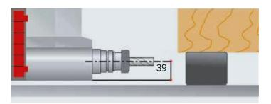
5-axis machining unit geometry allows it to operate at angles of up to 10° below the work piece supporting surface.
