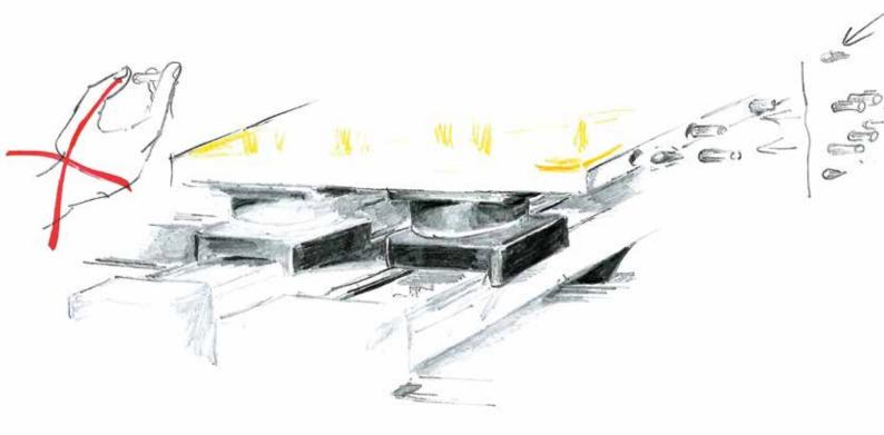
Optimization of productivity with no more time wasting for cleaning operations, thanks to the use of glue capsules, contrary to traditional dowelling devices where it is necessary to remove the remaining drying glue from the various components after a temporary production-stop.
