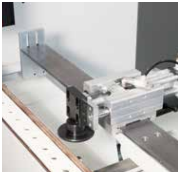
Device for semi-automatic feeding of workpieces for crosswise processing (option).
