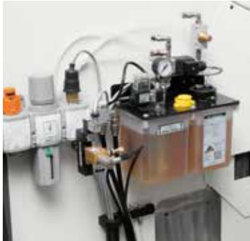
Automatic lubrication of the screw for the mobile beam positioning and of the transmission shaft screw of the feed chains.
