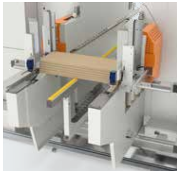
Manual hopper feeder for an higher productivity (option).
