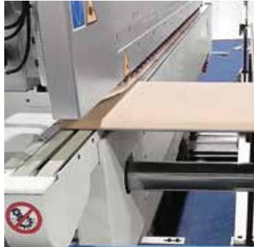
Motorized belts at machine outfeed to enable easy workpiece unloading (option).
