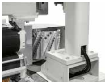
Trailing-edge profiling station Performs the profiling of panels up to 200 mm thick in a single pass, in two passes for thicknesses from 200 to 400 mm.
